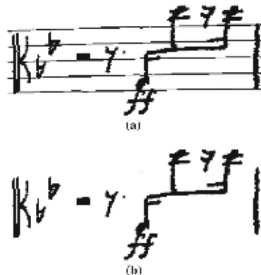
Fig. 5 Example of a staff removal process using SVM classifier, 81 features per pixel and only one condensed score as training set. a Input score. b Score after staff removal
